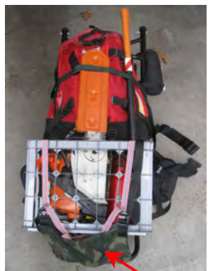
Straps and nylon cloth “shelf” stabilize crate and support handle of saw hanging through hole in crate bottom. Gas, oil and leaky saw are completely outside the pack.
