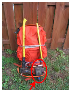
Saw body visible in red oval. Bar is slipped under pack. “Shelf” made of metal tubing supports saw body and other tools. Balanced and sturdy. Photo by Mark Cumnock.
