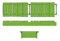
the lath yet applied, are *shown above.* "Decking" is pressure-treated 2x4's, usually 36" wide.
