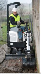
Left: Bobcat 1418 Compact Excavator, for grading & trenching. Rubberized treads minimize impact on trail tread.
