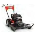
Left: DR Mower – Hand-driven, maneuverable brush-hog that can quickly put a clump of multiflora roses in its place. Uses: To clear or mow trail corridor. Newer models can be operated by smaller sized folks pretty easily. Can be stowed in a FLTC covered tool trailer and towed behind a sedan.
