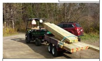
Nova Jack Woods Trailer – Double axel trailer has sides (above, flush with tires) that can be removed so arms (below, yellow) can hold a more narrow or longer load. Manueverable enough to use on jeep roads or temporary "service trails," towed behind an ATV or UV. Empty trailer is road-ready and easily towed behind a van, truck, small SUV, or Subaru Outback.
